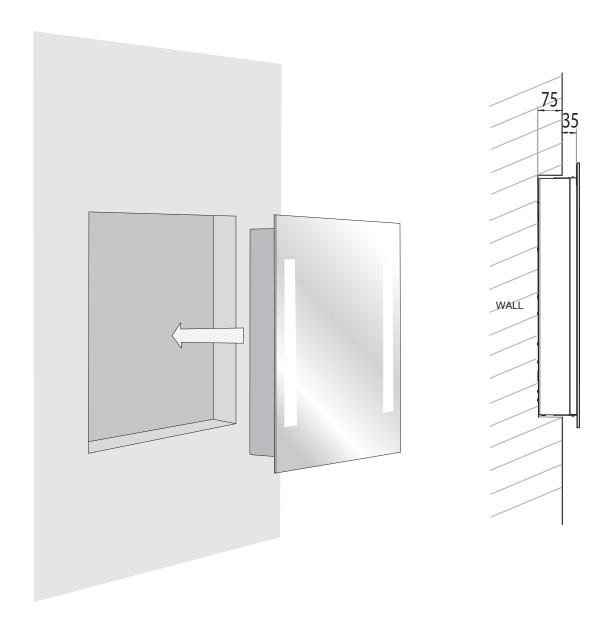
**N.B.** If the Livorno shaver cabinet is recessed, the shaver socket will not be usable for the charging of re-chargeable appliances. This is because the removeable switch cannot not be utilised if the cabinet is recessed.
